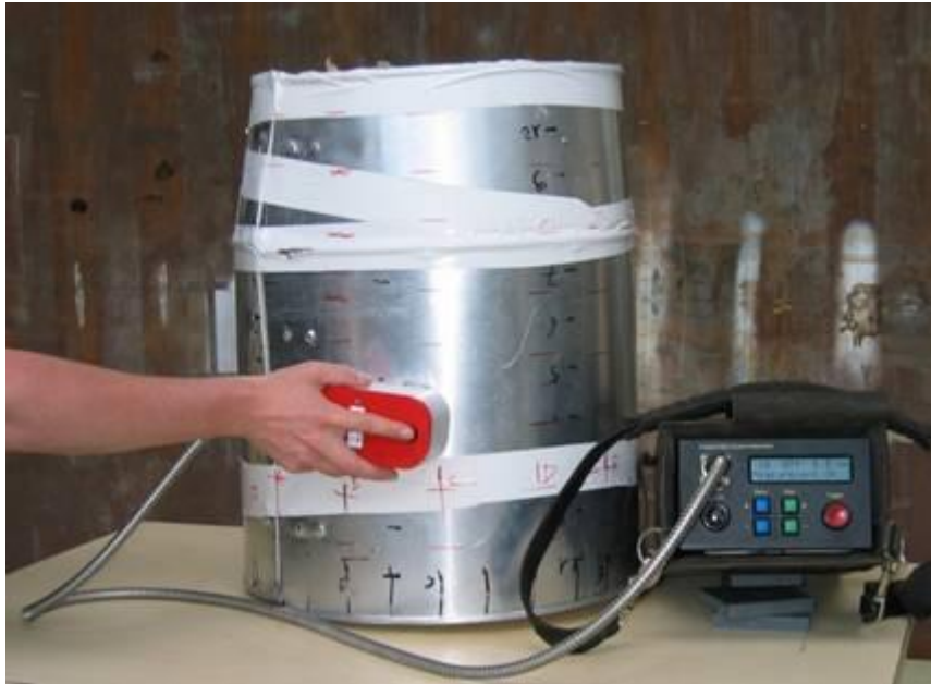
Insulated test sample with FAC examined by PEC
