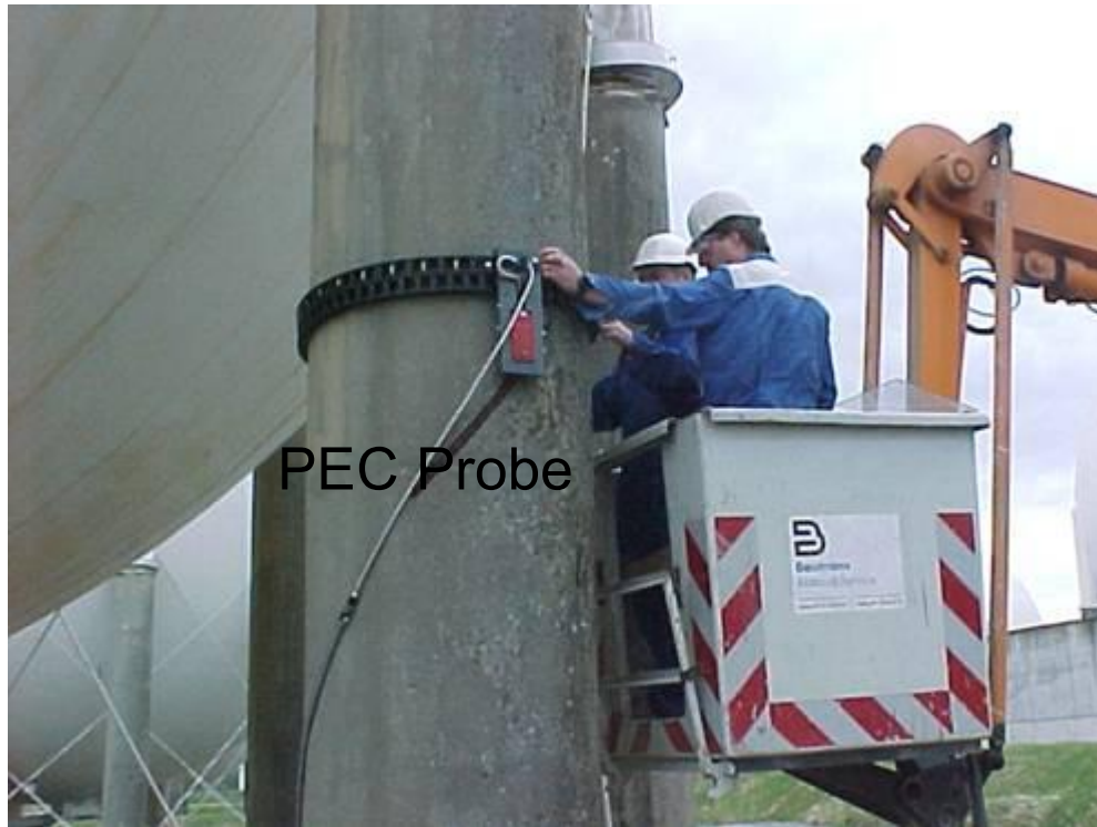
PEC probe in jig operated from cherry picker
