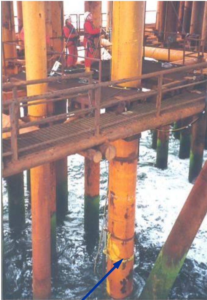
Jig with PEC probe
